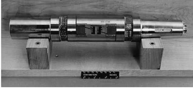
Fig. 1 Typical six-degree-of-freedom internal wind-tunnel force balance.
